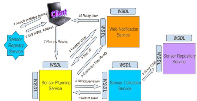
Fig. 3: A typical invocation for Sensor Web client.
