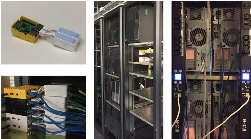
Figure 2. The CLOUDS-Pi platform. The top-left image shows a Raspberry Pi in an enclosure with four TP-Link USB-to-Ethernet adapters connected to available USB ports. The bottom-left image illustrates the 10 Raspberry Pi switches in a fat-tree-like topology. The middle image shows CLOUDS-Pi’s tower servers in the racks. The right image shows the two Eaton ePDU (enclosure power distribution units) for power monitoring and management.
