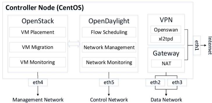
Figure 3. The software stack on the controller node. VM = virtual machine, VPN = virtual private network, eth = Ethernet interface, and NAT = network address translation.
