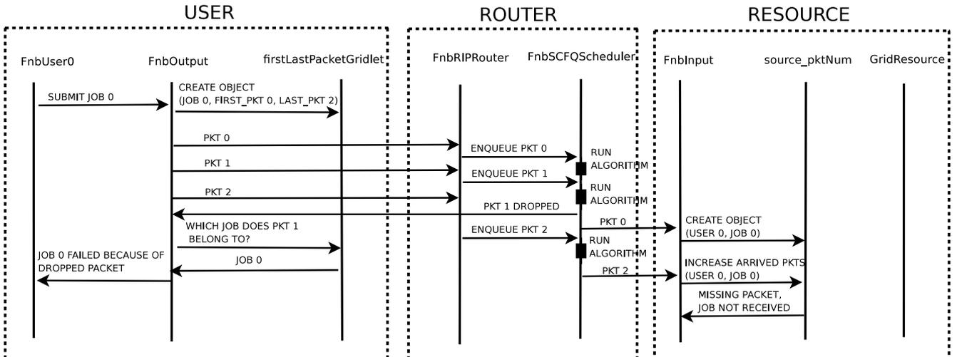
Figure 3. Sequence diagram showing a transmission with one dropped packet.
