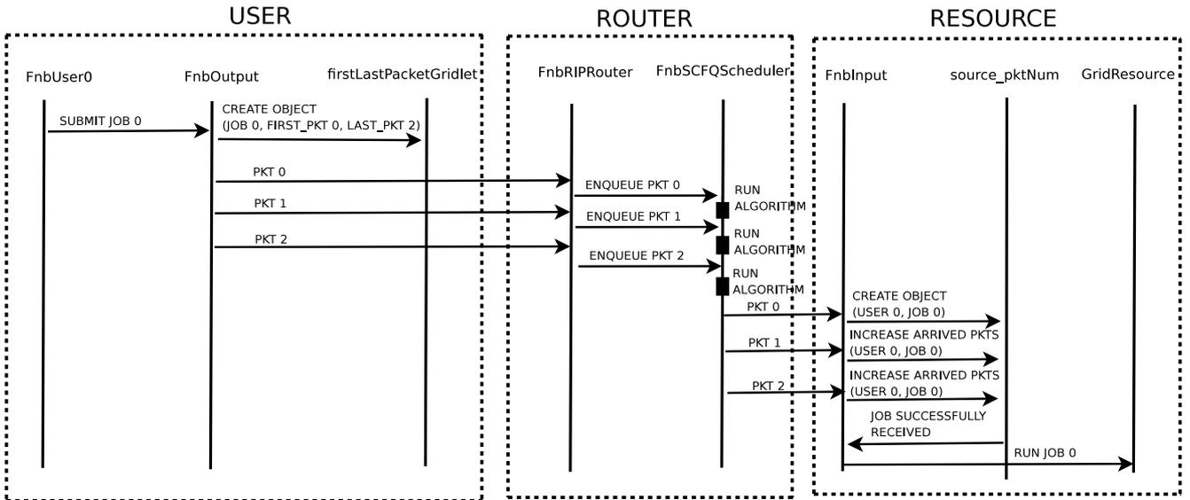
Figure 2. Sequence diagram showing a transmission with no dropped packets.
